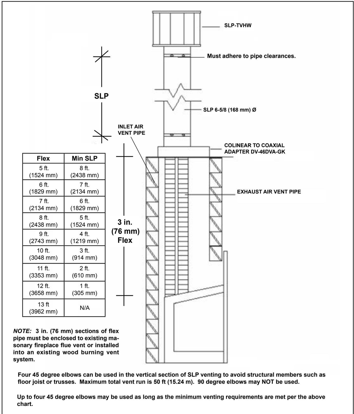
Figure 5.11 Optional SLP Venting Configuration - Vertical Termination
