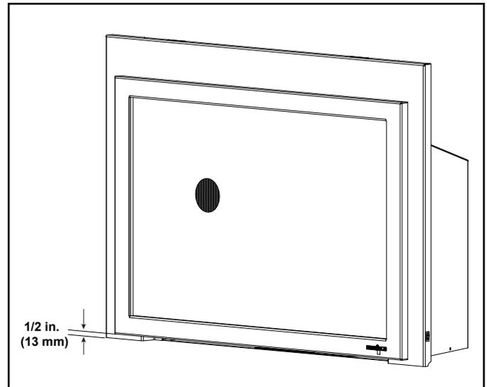
Figure 3.5 Minimum Required 1/2 in. (13 mm) Gap
