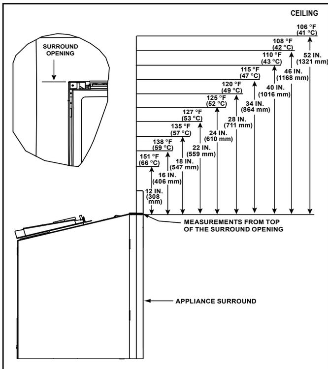
Figure 2.4 Good Faith Wall Surface Temperatures Above Appliance
