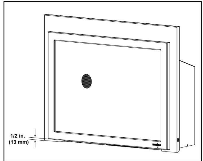
Figure 9.5 Required 1/2 in. (13 mm) Gap
