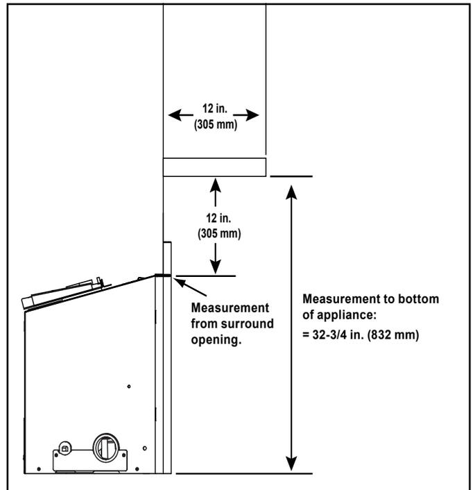
Figure 3.13 Minimum Vertical and Maximum Horizontal Dimensions - Combustible
