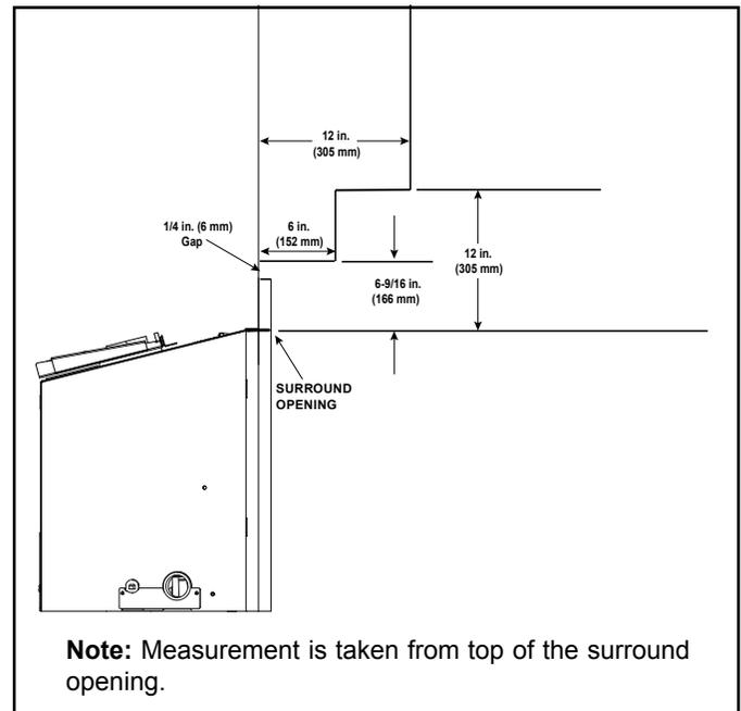
Figure 8.2 Minimum Vertical and Maximum Horizontal Dimensions - Non-Combustible
